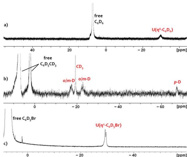
Fig. 5  $^2\text{H}$  NMR spectra of (a)  $2\text{-d}_6$  in  $\text{C}_6\text{H}_5\text{Br}$  containing 5 equiv. of  $\text{C}_6\text{D}_6$ , (b)  $3\text{-d}_8$  in  $\text{C}_6\text{H}_5\text{Br}$  containing 5 equiv. of toluene- $\text{d}_8$ , and (c)  $4\text{-d}_5$  in neat  $\text{C}_6\text{D}_5\text{Br}$ .
