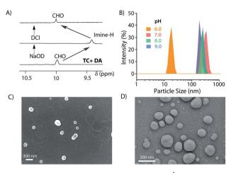
**Fig. 2** Formation of the SPA vesicles. (A) Partial <sup>1</sup>H-NMR showing formation/disruption of the imine linked SPAs, (B) DLS profile of assemblies formed at different pH values, (C) FESEM, and (D) FETEM images of the vesicles formed at pH 8.
