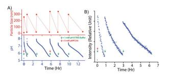
Fig. 7 (A) Time dependent variation in pH (bottom) and particle size (top) across six consecutive pH cycles. Note: 1 mM pH 9 TRIS buffer was added to 100 µM nanozyme solution to initiate each cycle and 5 mM pNPCAA was added before initiating the 1st and 4th cycles. (B) Fluorescence kinetics across three consecutive cycles using the DPH lipophilic probe. [DPH] = 10  $\mu$ M,  $\lambda_{ex}$  (DPH) = 355 nm,  $\lambda_{em}$  (DPH) = 428 nm.
