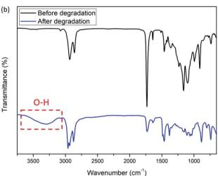
Fig. 3 Degradation of poly(ether-alt-ester). GPC trace (a, top) and FTIR spectra (b, bottom) of poly(ether-alt-ester) and degradation products (condition: 0.1 M tetrabutylammonium hydroxide in MeOH/DCM, room temperature, 2 h).
