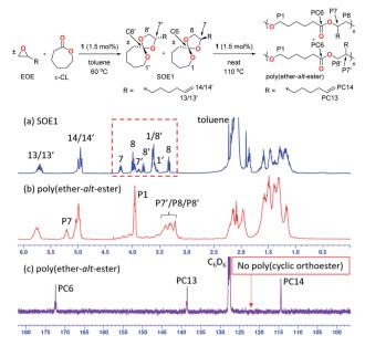
Fig. 1 One-pot synthesis of poly(ether-alt-ester) (Table 1, entry 1).  $^1$ H NMR spectra of (a) crude intermediate product of SOE1, (b) poly(ether-alt-ester), and (c)  $^{13}$ C{ $^1$ H} NMR spectrum of poly(ether-alt-ester) (400 MHz,  $C_6D_6$ , 25  $^{\circ}$ C).
