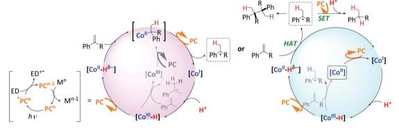
Scheme 5 Possible mechanistic scenarios for the reduction of aromatic olefins by the light-driven dual-copper-cobalt catalytic system in aqueous media. The highlighted  $[Co^{II}]$  intermediate indicates the beginning of the catalytic cycle. Acronyms stand for PC = photoredox catalyst; ED = electron donor; SET = single electron transfer and HAT = hydrogen atom transfer.
