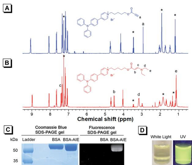
Fig. 2 <sup>1</sup>H NMR spectra of (A) TPAP-C5-yne and (B) TPAP-C5-aa in CDCl<sub>3</sub>. The solvent peaks are marked with asterisks. (C) SDS-PAGE gels showing protein bands of BSA and BSA-TPAP-C5-yne on coomassie blue (left) and fluorescence (right). (D) Photographs of BSA-TPAP-C5-yne aqueous dispersion under white light (left) and UV irradiation (right).
