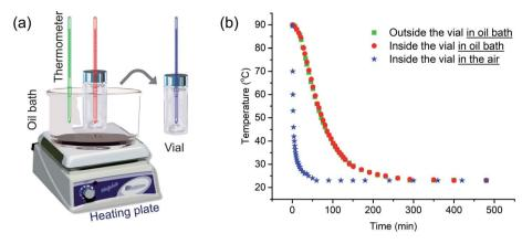
Fig. 1 (a) A representative simple equipment for block copolymer self-assembly. For cooling in the air, the vial was heated in the oil bath first and then taken out for cooling. (b) Temperature changes vs. time during cooling procedure.
