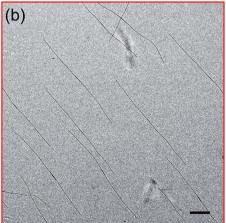
Fig. 3 TEM images of micelles formed via co-self-assembly of PFS<sub>45</sub>/PFS<sub>48</sub>-b-PI<sub>325</sub> (1 w/w%) in decane (1 mg mL $^{-1}$ ) under different cooling protocols. Both samples were heated at 90 °C for 30 min then cooled to 23 °C: (a) quick cooling; (b) slow cooling. Scale bars: 1  $\mu$ m.
