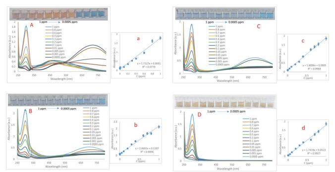
Fig. 2 The UV-Vis spectra of (A) AgNPrs, (B) Cys-capped AgNPrs, (C) Met-capped AgNPrs and (D) AgNWs sensing probes and calibration curves in the presence of various concentration of arsenic (0.0005, 0.001, 0.005, 0.01, 0.05, 0.1, 0.2, 0.3, 0.4, 0.6, 0.7, 0.8 and 1 ppm).
