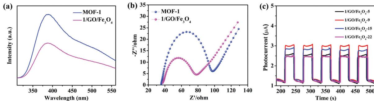
Fig. 8 (a) Photoluminescence spectra of **MOF-1** and  $1/\text{GO}/\text{Fe}_3\text{O}_4$ -9 (solid, temperature:  $25 \text{ }^\circ\text{C}$ ). (b) EIS Nyquist impedance plots of **MOF-1** and  $1/\text{GO}/\text{Fe}_3\text{O}_4$ -9. (c) Transient photocurrent responses of the  $1/\text{GO}/\text{Fe}_3\text{O}_4$  composite.
