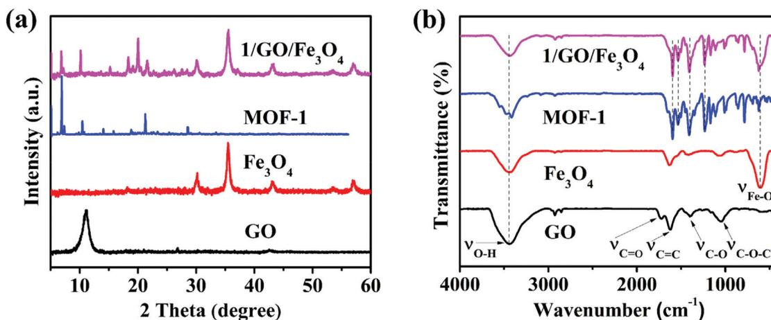
**Fig. 2** PXRD patterns (a) and FT-IR spectra (b) of GO,  $\text{Fe}_3\text{O}_4$ , MOF-1, and 1/GO/ $\text{Fe}_3\text{O}_4$  (solid, temperature: 25 °C).
