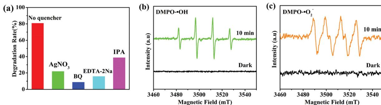
Fig. 7 (a) Effect of different scavengers on the photodegradation of chlortetracycline over  $1/\text{GO}/\text{Fe}_3\text{O}_4$ -9. ESR spectral investigation of the produced  $\cdot\text{OH}$  (b) and  $\cdot\text{O}_2^-$  (c) in the dark and after light radiation for 10 minutes ( $1/\text{GO}/\text{Fe}_3\text{O}_4$  concentration:  $0.45 \text{ g L}^{-1}$ ,  $\text{H}_2\text{O}_2$  concentration:  $10 \text{ mM}$ , temperature:  $25 \text{ }^\circ\text{C}$ ).
