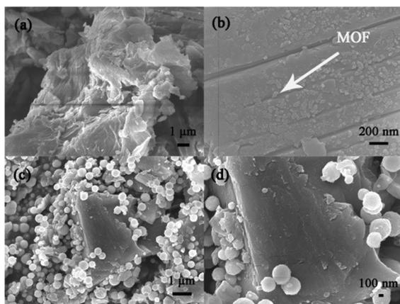
Fig. 3 SEM images of MOF-1/GO (a and b) and 1/GO/Fe<sub>3</sub>O<sub>4</sub> (c and d).
