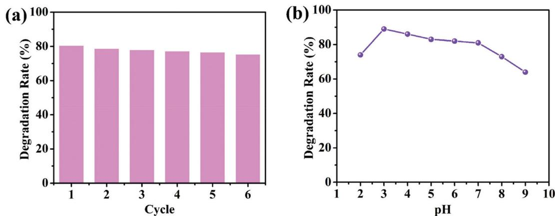
**Fig. 6** (a) Recycling tests for the degradation of chlortetracycline by the 1/GO/Fe<sub>3</sub>O<sub>4</sub>-9 composite. (b) Effects of the initial pH on the degradation of chlortetracycline.
