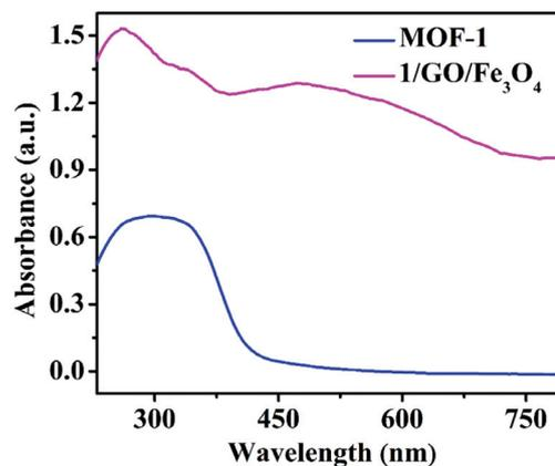
Fig. 4 UV-Vis diffuse reflectance spectra of MOF-1 and the 1/GO/Fe<sub>3</sub>O<sub>4</sub> composite (solid, temperature: 25 °C).
