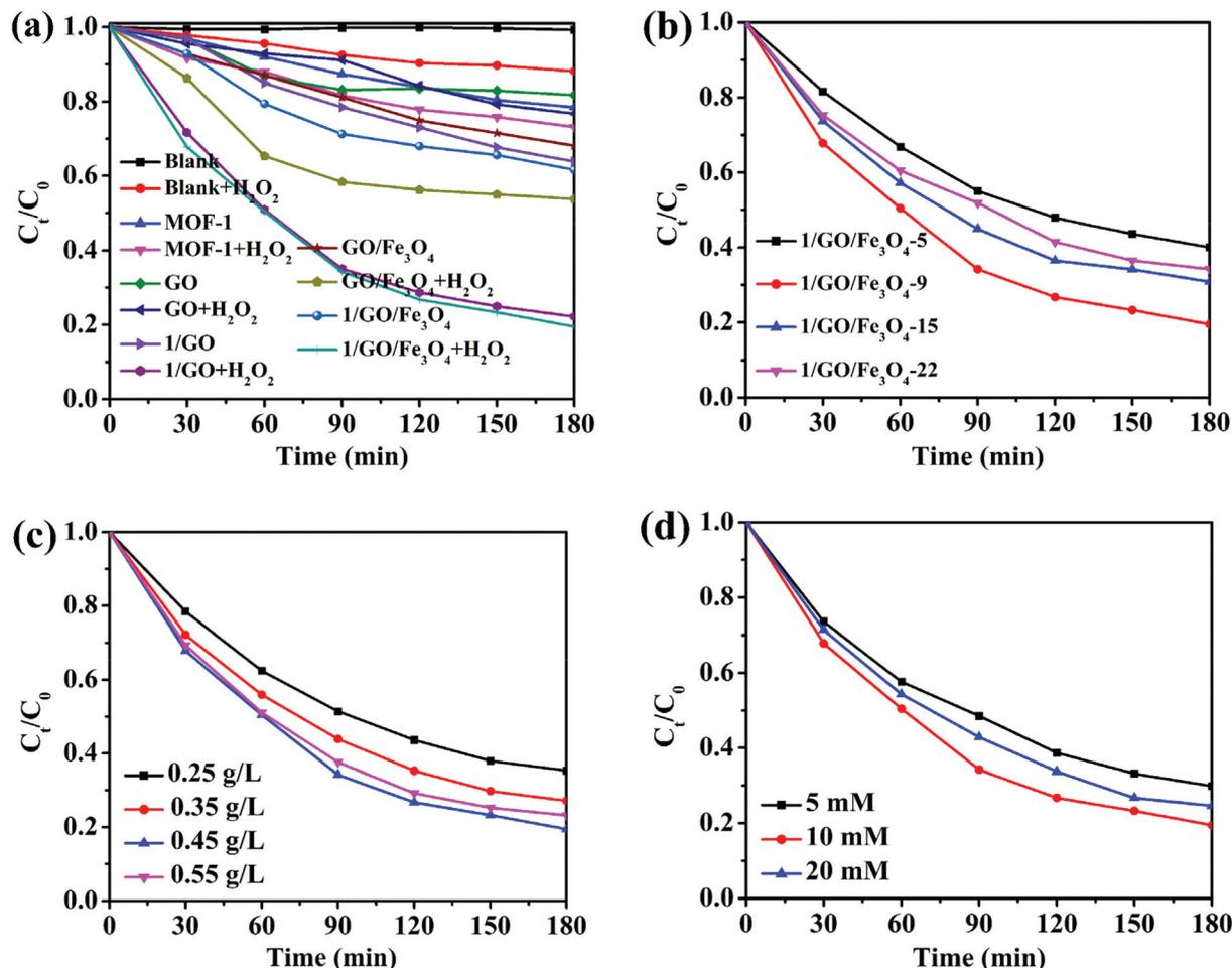
Fig. 5 (a) Photocatalytic degradation efficiency of chlortetracycline over different photocatalysts. Influence of the (b) GO content, (c) catalyst concentration, (d) H<sub>2</sub>O<sub>2</sub> concentration on the degradation of chlortetracycline (except for the investigated parameter, other parameters were set as follows: 20 mg L<sup>-1</sup> chlortetracycline, 0.45 g L<sup>-1</sup> 1/GO/Fe<sub>3</sub>O<sub>4</sub>, and 10 mM H<sub>2</sub>O<sub>2</sub>).
