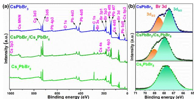
Fig. 3 (a) Wide-scan X-ray photoelectron spectrum of emissive  $\text{CsPbBr}_3$ , dual-phase  $\text{CsPbBr}_3/\text{Cs}_4\text{PbBr}_6$  and non-emissive  $\text{Cs}_4\text{PbBr}_6$ . (b) High-resolution X-ray photoelectron spectra of Br (3d).
