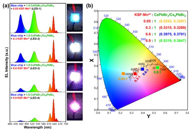
Fig. 9 (a) The electroluminescence spectra of the designed LED devices by varying the K<sub>2</sub>SiF<sub>6</sub>:Mn<sup>4+</sup> to CsPbBr<sub>3</sub>/Cs<sub>4</sub>PbBr<sub>6</sub> ratio in the wt% of 0.05:1, 0.3:1, 0.6:1, and 0.9:1 under forward-bias current of 20 mA (inset images are photographs of the working LEDs (LED 1–4)), (b) the CIE chromaticity coordinates corresponding to the constructed LED devices using different composite wt% ratios.
