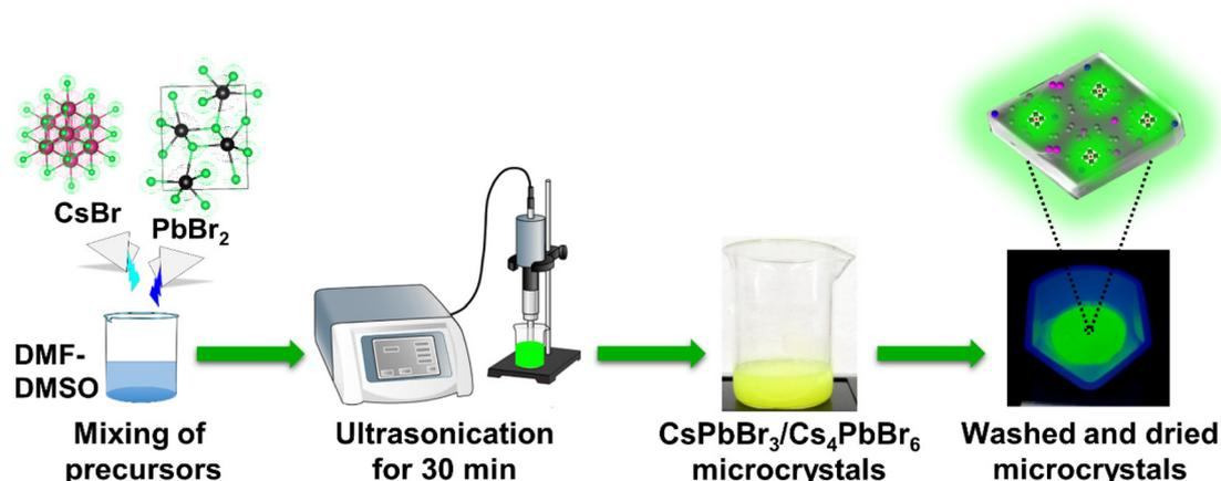
Fig. 1 Scheme for the synthesis of dual-phase CsPbBr<sub>3</sub>/Cs<sub>4</sub>PbBr<sub>6</sub> MCs using ultrasonication process.
