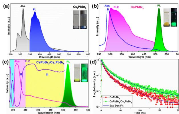
Fig. 5 (a) Absorption and photoluminescence spectra of pure Cs<sub>4</sub>PbBr<sub>6</sub>, (b) absorption, photoluminescence, and excitation spectra of pure CsPbBr<sub>3</sub>, (c) absorption, photoluminescence, and excitation spectra of dual-phase CsPbBr<sub>3</sub>/Cs<sub>4</sub>PbBr<sub>6</sub>, and (d) time-resolved photoluminescence decay curves of CsPbBr<sub>3</sub>, and CsPbBr<sub>3</sub>/Cs<sub>4</sub>PbBr<sub>6</sub> at  $\lambda_{\text{exci}} = 365$  nm.
