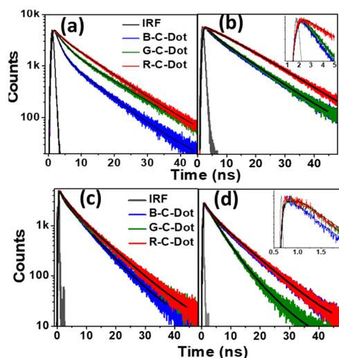
**Fig. 2** Time-resolved PL decay of the C-Dots monitored at (a) 440 nm and (b) 530 nm after excitation at 340 nm, and at (c) 440 nm and (d) 530 nm after 405 nm excitation (inset: zoomed data at the earlier time scale).
