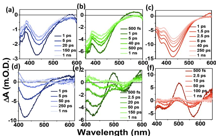
**Fig. 3** TA spectra of the (a) B-C-Dots, (b) G-C-Dots, and (c) R-C-Dot at different time delays after 320 nm excitation. TA spectra of the (d) B-C-Dots, (e) G-C-Dots, and (f) R-C-Dots at different time delays after 380 nm excitation.
