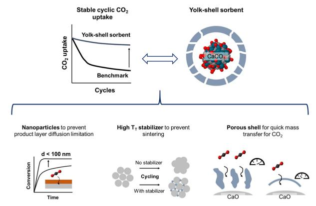
Fig. 1 Design approach for yolk–shell-type CaO-based sorbents. Using a nanoparticle core is expected to prevent diffusive limitations due to product layer formation, whereas a porous shell of a high  $T_T$  stabilizer shall mitigate sintering of the nanoparticles while at the same time allowing for a rapid transfer of CO<sub>2</sub> to unreacted CaO.
