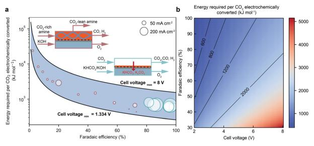
Fig. 6 (a) A comparison of the energy consumption, CO faradaic efficiency, and cell potentials over integrated and gas-fed  $CO_2$  electrolysis. (b) The role of CO faradaic efficiency and cell voltage in determining the overall energy consumption of  $CO_2$  electrolysis to produce  $CO_2$ .
