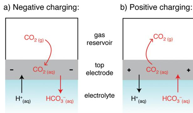
Fig. 3 Schematic showing the proposed mechanism for the movement of CO<sub>2</sub> and ions with charging. Other cations (*e.g.* Na<sup>+</sup>) will behave analogously to H<sup>+</sup>, and anions (*e.g.* CO<sub>3</sub><sup>2-</sup> and Cl<sup>-</sup>) to HCO<sub>3</sub><sup>-</sup>.
