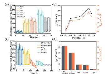
Fig. 8 (a) The amperometric I-t curves of HV-SnS<sub>2</sub>/MoS<sub>2</sub> under different bias voltages. (b)  $I_{ph}$  and  $R_{ph}$  of HV-SnS<sub>2</sub>/MoS<sub>2</sub> as a function of bias voltage. (c) The amperometric I-t curves of different photoelectrodes under 0.8 V. (d)  $I_{ph}$  and  $R_{ph}$  of different photoelectrodes under 0.8 V.
