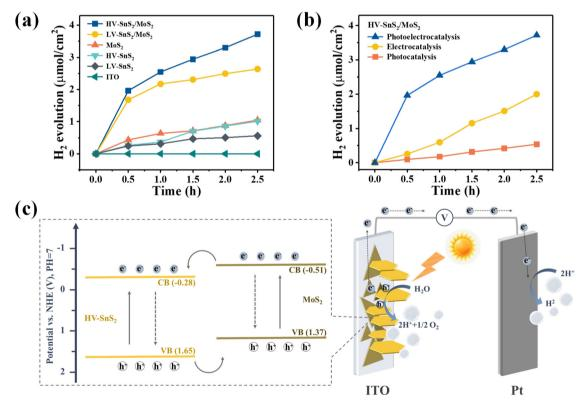
Fig. 9 (a) Photoelectrocatalytic  $H_2$  production of different photoanodes in 1 M  $H_2SO_4$  under 0.8 V. (b) Photocatalytic (100 mW cm<sup>-2</sup>), electrocatalytic (0.8 V), and photoelectrocatalytic (100 mW cm<sup>-2</sup>, 0.8 V)  $H_2$  production of  $HV-SnS_2/MoS_2$  photoanode. (c) The schematic plot of charge transfer pathways in  $HV-SnS_2/MoS_2$  heterostructure as an effective photoelectrode for PEC water splitting.
