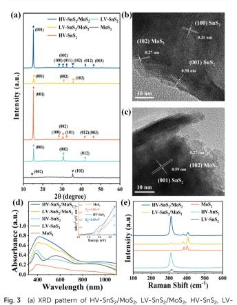
$SnS_2$ , and  $MoS_2$ . (b) TEM image of HV- $SnS_2/MoS_2$ . (c) TEM image of LV-SnS<sub>2</sub>/MoS<sub>2</sub>. (d) UV-Vis absorption spectroscopy of all samples. The inset is Tauc plot for estimating the bandgap energies ( $E_{q}$ ) of MoS<sub>2</sub> and HV-SnS<sub>2</sub>. (e) Raman spectra of all samples.
