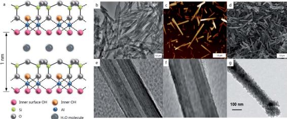
Fig. 1 Schematics of the tube wall composition (a), and TEM, AFM and SEM images of pristine halloysite nanotubes, the samples provided by Applied Minerals Inc, USA, (b–d) and TEM images of increasing halloysite lumen diameter from 12 to 25 nm with sulphuric acid etching (e and f); the nanotube LbL-coated with (polyethyleneimine/7 nm silica)<sub>2</sub> shell (g), adapted from ref. 7 with permission from Wiley, copyright 2016.
