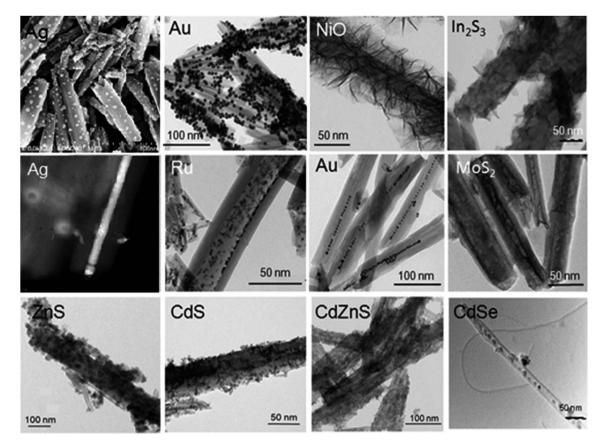
Fig. 2 Metal containing core—shell structures based on clay nanotubes, upper row – location outside: Ag, Au, NiO, and  $In_2S_3$  – taken from ref. 29 with permission, copyright by Elsevier, 2015. Middle row – tubes loaded inside: Ag, Ru, Au, and MoS<sub>2</sub>; bottom row – halloysite loaded inside/outside: ZnS, CdS, CdZnS, and CdSe.
