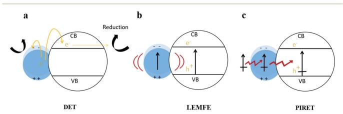
Fig. 8 Energy transfer mechanism in metal/semiconductor structures. Reprinted from ref. 103. Copyright 2012, ACS.
