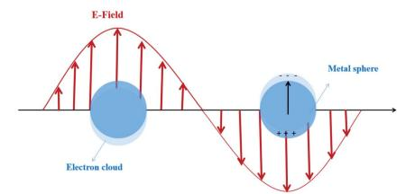
Fig. 2 Local surface plasmon resonance excitation. Reprinted from ref. 13. Copyright 2014, ACS.
