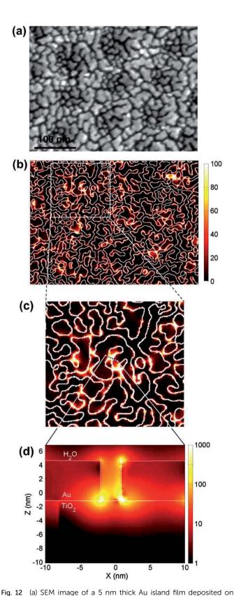
anodic TiO<sub>2</sub>. (b–d) Electric field intensities calculated at the interface of Au–TiO<sub>2</sub> using the FDTD method. Reprinted from ref. 104. Copyright 2011 Elsevier.
