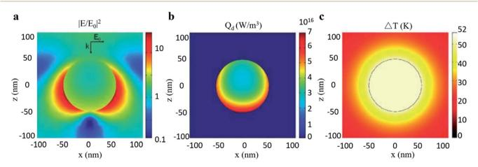
Fig. 14 Photothermal effect of a gold sphere with 50 nm radius in water. (a) Electric field intensity normalized to the incident field. (b) Heat power volume density  $Q_d$ . (c) Steady-state temperature increase due to 530 nm light excitation. Reprinted from ref  $^{30}$ . Copyright 2012 American Chemical Society.
