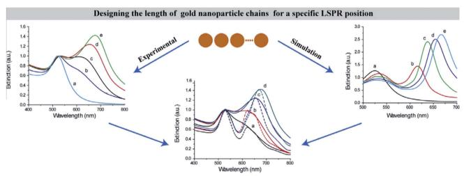
"Trial and error" fit of the experimental data with a linear combination of numerical simulations
