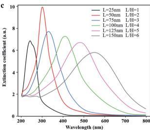
Fig. 3 Highly controllable optical properties of LSPR. (a) Absorption spectra of composite glass with different contents of Ag nanoparticles. Reprinted from ref. 21. Copyright 2005, Springer. (b) Normalized extinction of Au@SnO $_2$  with varying structures. Reproduced with data source from ref. 24. (c) Extinction coefficient spectra of Al NPs of different sizes. Reproduced with data source from ref. 26.
