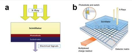
Fig. 1 (a) Schematic depiction of the three main functional layers in a common X-ray CT detector. Reproduced with permission.<sup>34</sup> Copyright 2013 Springer Nature Limited. (b) Schematic description of an X-ray flat detector constituted by columnar CsI:TI<sup>+</sup> scintillator and a detecting matrix of amorphous-silicon photodiodes. Reproduced with permission. 18 Copyright 2013 Elsevier.
