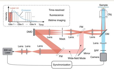
Fig. 1 Schematic diagram of the TR-SIM & TR-WF microscope. DMD, digital micromirror device; FM, flexible mirror; Obj, objective lens; DM, dichroic mirror; SPF: short pass filter. The inset (top left) illustrates the time-resolved fluorescence lifetime imaging from 0 µs to 3000 µs with a time-gate of 100  $\mu$ s and a gated excitation laser from 0  $\mu$ s to 200  $\mu$ s.
