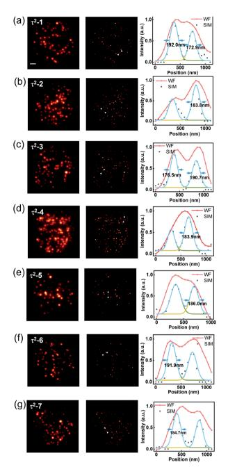
Fig. 4 Comparison of TR-WF and TR-SIM with seven kinds of  $\tau^2$  dots. For each group, TR-WF and TR-SIM and the line profiles of selected areas (indicated by the arrows in TR-SIM images) are shown from left to right. Scale bar: 2 µm.
