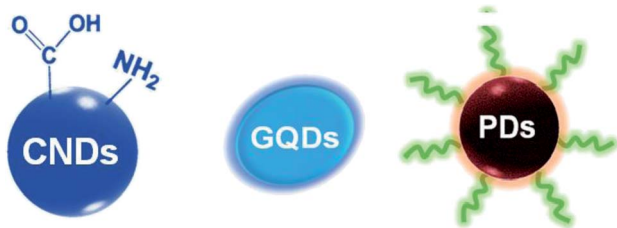
Fig. 2 Illustration of three different types of carbon dots (CDs), from left to right: carbon nanodots (CNDs), graphene quantum dots (GQDs) and polymer dots (PDs).
