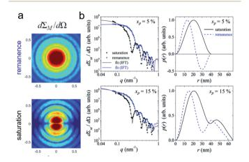
Fig. 16 Results of the micromagnetic SANS modelling for an ensemble of spherical Fe particles with a diameter of D=40 nm. (a) The total magnetic SANS cross-section in the perpendicular scattering geometry ( $x_p = 15\%$ ). (b) Azimutally-averaged total magnetic SANS cross-sections and corresponding distance distribution functions p(r)for  $x_p = 5\%$  and  $x_p = 15\%$ . Reprinted figure with permission from Vivas et al. 373 Copyright 2020 by the American Physical Society.
