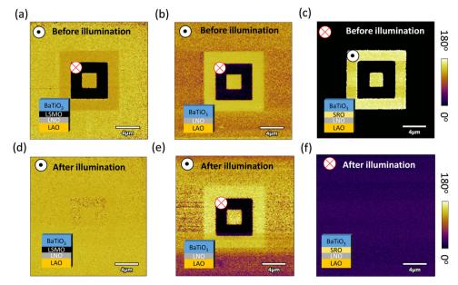
Fig. 3 PFM phase images collected (a-c) before and (d-f) after illumination for the BTO/LSMO, BTO/LNO and BTO/SRO samples, respectively
