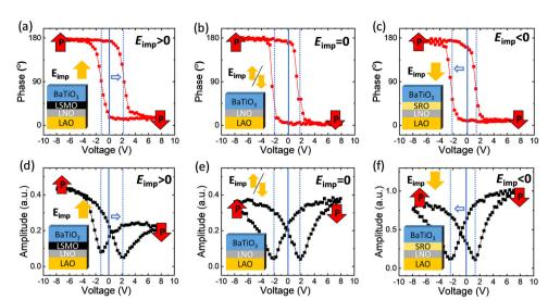
Fig. 2 (a-c) PFM phase and amplitude (d-f) loops of the BTO/LSMO, BTO/LNO and BTO/SRO samples, respectively. Sketches of the  $E_{imp}$  direction are indicated by vertical (yellow) and horizontal (open blue) arrows.
