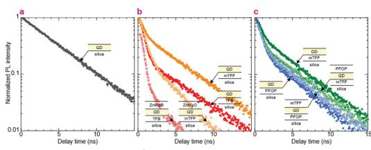
Fig. 4 Time-resolved photoluminescence decay. Mesolight<sup>®</sup> blue-QDs (20 nm thick film): (a) on fused silica, (b) on the polymer HTL, before and after deposition of ZnMgO nanoparticles, (c) on the polymer HTL or ETL, before and after the lay down of the opposite transport layer. The fast component comes primarily from the polymer ( $\tau \approx 0.7$  ns) and the slow component from the QDs ( $\tau \approx 4.3$  ns in pristine film). Excitation, 374 nm; emission, 465 nm.
