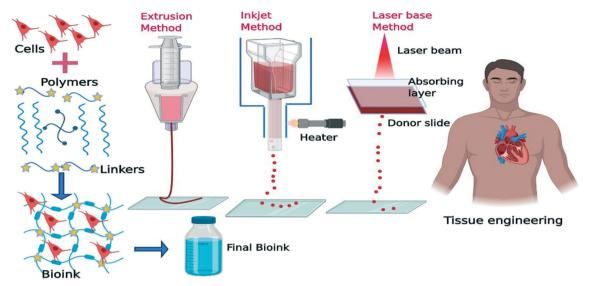
Fig. 4 Schematic illustration of the bio-printing process in tissue engineering applications (created with BioRender).
