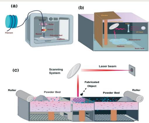
Fig. 2 Schematic representation of AM fabrication processes: (a) fused deposition modeling, (b) stereolithography and (c) selective laser melting<sup>48</sup> (created with BioRender).
