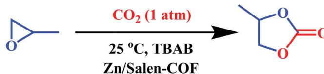
Fig. 17 Cycloaddition involving CO<sub>2</sub> and a terminal epoxide catalyzed by Zn-salen-COF-SDU113.
