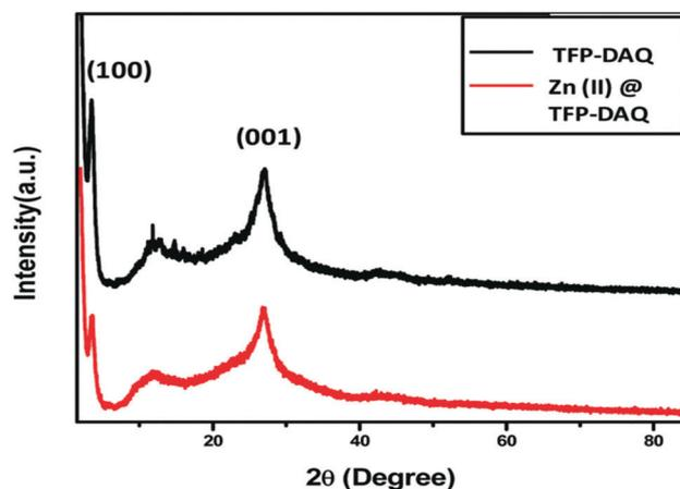
Fig. 19 The PXRD analysis of TFP-DAQ COF and Zn(II)@TFP-DAQ COF. Reproduced with permission from ref. 52; copyright: 2020, New Journal of Chemistry.
