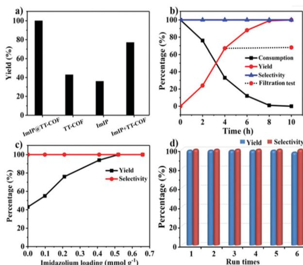
Fig. 15 (a) The catalytic activities of ImIP@TT-COF, ImIP, TT-COF, and a blend of imidazolium salt and TT-COF. (b) Kinetic curves for the CO<sub>2</sub> cycloaddition reaction. (c) The impact of ImIP content. (d) The recyclability of the COF. Reproduced with permission from ref. 40; copyright: 2020, ChemSusChem.
