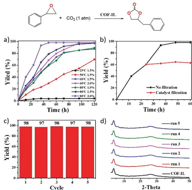
**Fig. 11** (a) The effects of temperature, reaction time, and catalyst amount on COF-IL-catalysed CO<sub>2</sub> cycloaddition to styrene oxide. (b) Reaction time analysis (black line) and leaching testing (red line) during CO<sub>2</sub> cycloaddition to styrene oxide catalyzed by COF-IL. (c) Recycling of the catalyst. (d) PXRD patterns from every catalytic cycle. Reproduced with permission from ref. 32; copyright: 2019, Journal of Materials Chemistry A.
