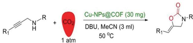
**Scheme 33** A general synthesis scheme for 2-oxazolidinones. Reproduced with permission from ref. 58; copyright: 2020, Journal of CO<sub>2</sub> Utilization.
