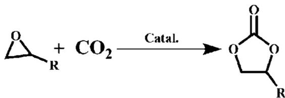
Scheme 17 The cycloaddition of CO<sub>2</sub> with substituted epoxides.
