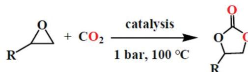
Scheme 6 The synthesis scheme for cycloaddition involving CO<sub>2</sub>. Reproduced with permission from ref. 22; copyright: 2020, ChemCatChem.
