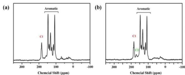
Fig. 5 (a) The solid-state <sup>13</sup>C-NMR spectrum of TpPa-Py-COF. (b) The solid-state <sup>13</sup>C-NMR spectrum of TpPa-Py-Br<sup>-</sup>-COF. Reproduced with permission from ref. 22; copyright: 2020, ChemCatChem.
