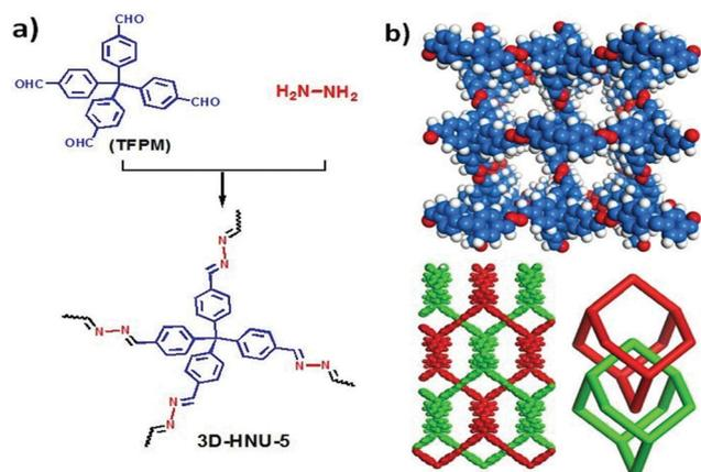
**Scheme 13** (a) The synthesis of 3D-HNU5 COF and (b) its 3D perforated structure and 2-fold interpenetrating diamond-like frame (blue: C, white: H, red: N). Reproduced with permission from ref. 29; copyright: 2019, Chemical Communications.
