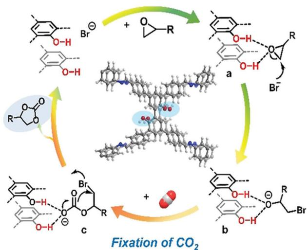
Scheme 19 A probable mechanism for CO<sub>2</sub> cycloaddition with ethylene oxides using methoxy-hydroxyl-TPBP-COF and tetrabutylammonium bromide. Reproduced with permission from ref. 39; copyright: 2020, Chemistry A European Journal.
