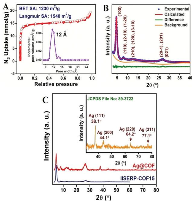
Fig. 4 (A) The  $\text{N}_2$  adsorption isotherm of IISERP-COF-15. (B) The PXRD pattern of the COF. (C) The PXRD pattern of Ag@COF. Reproduced with permission from ref. 21; copyright: 2019, Chemistry An Asian Journal.
