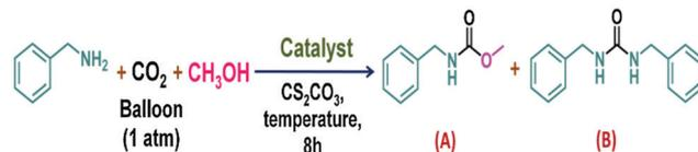
Scheme 28 Methyl benzyl carbamate synthesis *via* a CO<sub>2</sub> fixation reaction. Reproduced with permission from ref. 54; copyright: 2020, Molecular Catalysis.
