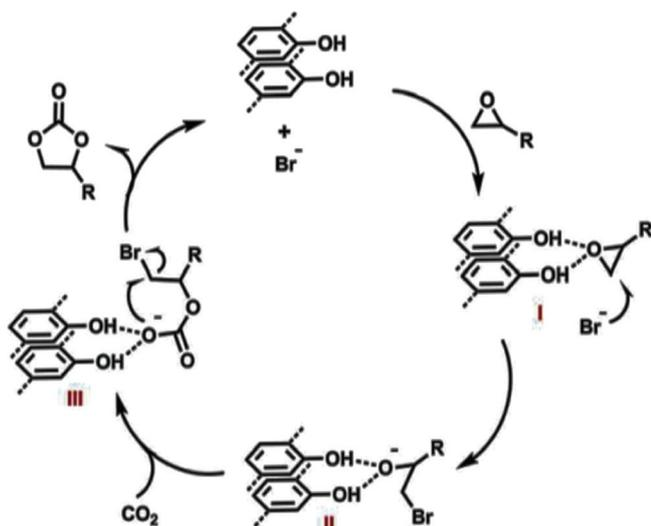
**Scheme 9** A self-explanatory mechanistic path supporting the cycloaddition of  $\text{CO}_2$  using COF-JLU7 and TBAB. Reproduced with permission from ref. 25; copyright: 2018, Journal of Materials Chemistry A.
