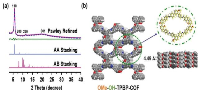
Fig. 14 (a) The powder XRD patterns of OMe-OH-TPBP-COF: experimentally observed (red), Pawley refinement (blue), and the difference (green), and simulations of AA-stacking (light blue) and AB-stacking (pink), (b) top and side views of OMe-OH-TPBP-COF. Reproduced with permission from ref. 39; copyright: 2020, Chemistry A European Journal.
