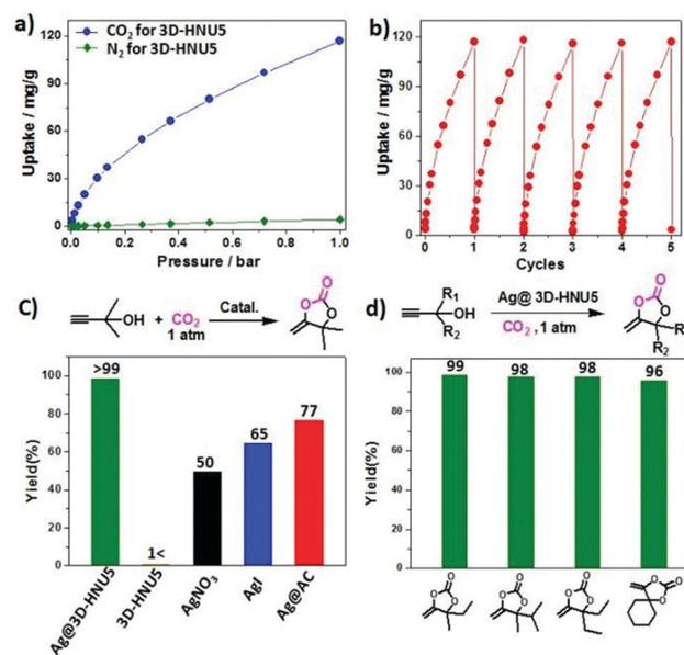
**Fig. 10** (a)  $\text{CO}_2$  and  $\text{N}_2$  isotherms for 3D-HNU5 COF at 273 K. (b)  $\text{CO}_2$  adsorption by 3D-HNU5 over multiple cycles at 273 K. (c) A study of catalysts for the formation of cyclic carbonates. (d) The yield percentages of different cyclic carbonates when Ag@3D-HNU5 is used as the catalyst. Reproduced with permission from ref. 29; copyright: 2019, Chemical Communications.
