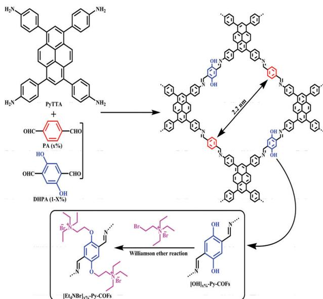
Scheme 1 The fabrication of [HO]<sub>X%</sub>-Py-COFs along with [Et<sub>4</sub>NBr]<sub>X%</sub>-Py-COFs.
