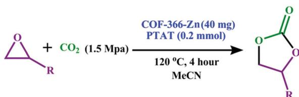
**Scheme 7** The synthesis of cyclic carbonates *via* CO<sub>2</sub> incorporation using COF-366-Zn. Reproduced with permission from ref. 23; copyright: 2017, Dalton Transactions.
