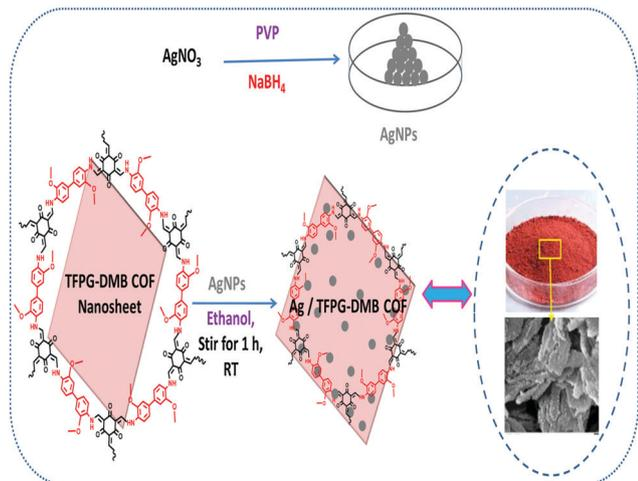
Scheme 27 The synthesis of Ag/TFPG-DMB COF. Reproduced with permission from ref. 54; copyright: 2020, Molecular Catalysis.
