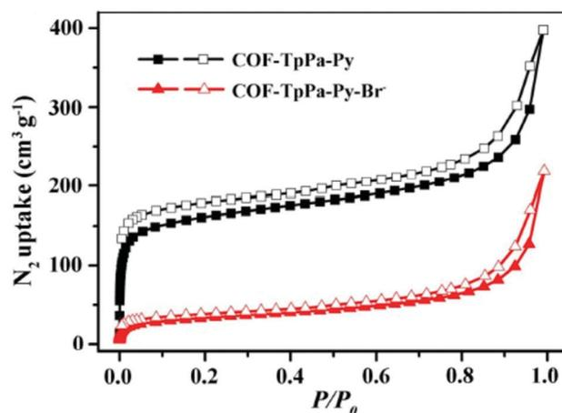
Fig. 7 The N<sub>2</sub> adsorption isotherm of TpPa-Py-Br<sup>-</sup>-COF. Reproduced with permission from ref. 22; copyright: 2020, ChemCatChem.
