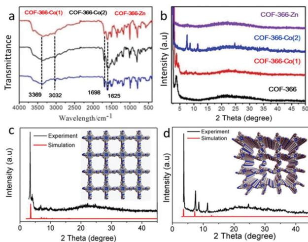
**Fig. 8** (a) FTIR and (b) PXRD analysis of COF-366-M catalysts, and PXRD patterns of (c) COF-366-Co(2) and (d) COF-366-Co(1). Reproduced with permission from ref. 23; copyright: 2017, Dalton Transactions.
