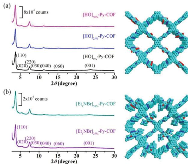
Fig. 2 Powder X-ray diffraction analysis of (a) [HO]<sub>X%</sub>-Py-COFs (where X is 0, 25, and 50) and (b) [Et<sub>4</sub>NBr]<sub>X%</sub>-Py-COFs (where X is 25 and 50). Top views of [HO]<sub>50%</sub>-Py-COF and [Et<sub>4</sub>NBr]<sub>X%</sub>-Py-COF (X = 50) are given in the right-side panels. Reproduced with permission from ref. 18; copyright: 2016, Chemical Communications.
