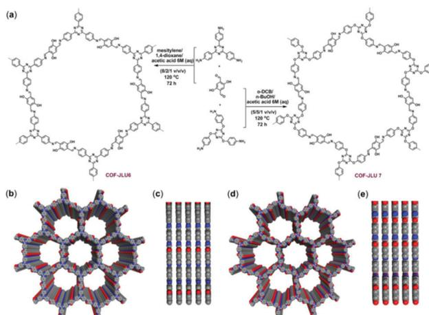
**Fig. 9** (a) A diagram of the synthesis of COF-JLU6 and COF-JLU7 *via* condensation. (b) Top and (c) side views of [COF-JLU6]. (d) Top and (e) side views of [COF-JLU7]. Reproduced with permission from ref. 25; copyright: 2018, Journal of Materials Chemistry A.
