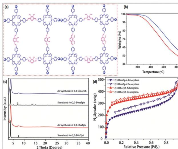
**Fig. 23** (a) The structure of a catechol-porphyrin COF; (b) TGA plots of (blue) 2,3-DhaTph and (red) 2,3-DmaTph; (c) PXRD analysis; and (d)  $\text{N}_2$ -BET analysis. Reproduced with permission from ref. 64; copyright: 2016, Catalysis Science & Technology.
