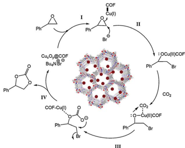
**Scheme 12** A probable mechanistic path for the synthesis of styrene carbonate *via* a cycloaddition reaction using the  $\text{Cu}_x\text{O}_y\text{@COF}$  catalyst and TBAB as a co-catalyst. Reproduced with permission from ref. 26; copyright: 2019, Journal of  $\text{CO}_2$  Utilization.
