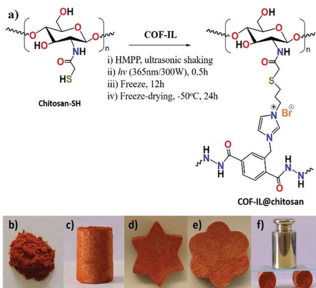
**Scheme 15** (a) The synthesis of COF-IL@chitosan. Photographs of (b) COF-IL (solid-crystals) and (c–e) COF-IL@chitosan (aerogel) with different shapes. (f) The pressure testing of an aerogel column done with a weight of 250 g. Reproduced with permission from ref. 32; copyright: 2019, Journal of Materials Chemistry A.
