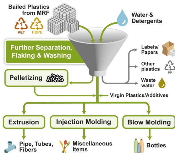
Fig. 13 Various approaches for mechanical recycling of PSW (plastic solid waste). 136
