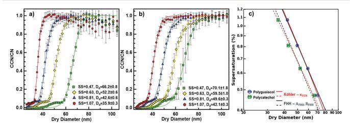
Fig. 2 CCN measurements and analysis. CCN/CN activation versus particle dry diameter for (a) polycatechol and (b) polyguaiacol at 4 different supersaturations. Each sigmoid fit (solid line) is the best fit average of 10 measurements. Error bars are standard deviation. (c) Köhler theory (red lines) and FHH model-based power law fits (black lines) of the CCN activity measurements of polycatechol and polyguaiacol. The derived FHH parameters can also be applied to subsaturated measurements.
