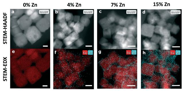
Fig. 1 (a-d) STEM-HAADF and (e-h) STEM-EDX images in as-prepared state for (a and e) pure  $Cu_2O$  NCs and bimetallic CuZn NCs with (b and f) 4% Zn. (c and g) 7% Zn and (d and h) 15% Zn. The white scale bars indicate a length of 20 nm.
