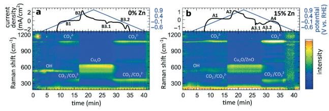
Fig. 9 Time-dependent SERS band intensities during the CV scan, and the corresponding changes in the current density for (a) pure Cu<sub>2</sub>O NCs and for the (b) Zn/Cu<sub>2</sub>O catalyst with a 15% Zn loading
