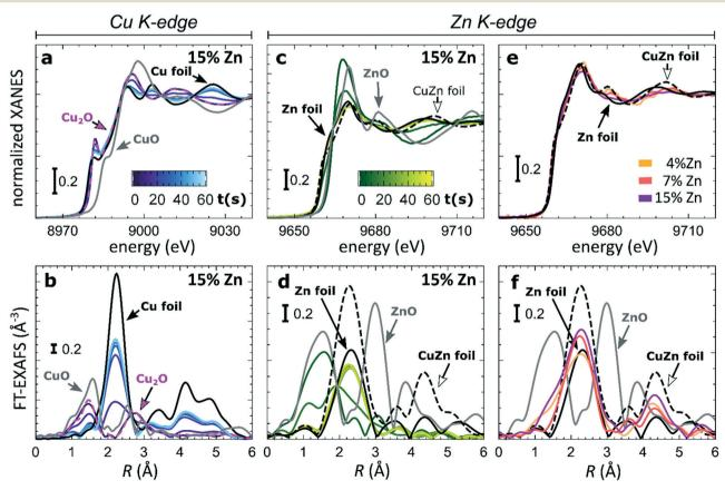
Fig. 3 The evolution of XANES and Fourier-transformed (FT) EXAFS spectra (a and b) at the Cu K-edge, (c and d) and the Zn K-edge during the first minute of CO<sub>2</sub>RR at -500 mA cm<sup>-2</sup>. (e and f) The final XANES and FT-EXAFS spectra at the Zn K-edge after 1 hour of CO<sub>2</sub>RR.
