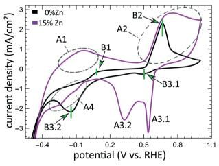
Fig. 7 Cyclic voltammogram for the Cu<sub>2</sub>O and bimetallic Zn/Cu<sub>2</sub>O catalysts with different Zn loadings. The current density is plotted as a function of the potential. The CV peaks for the bimetallic CuZn samples are labelled as A1, A2, A3.1, A3.2, and A4, while the CV peaks appearing in the pure Cu<sub>2</sub>O catalyst are denoted as B1, B2, B3.1, and B3.2.
