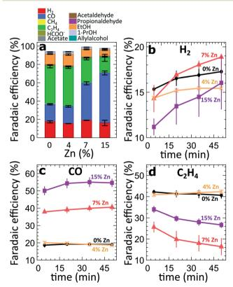
Fig. 2 (a) FEs of all catalysts after 50 minutes of  $CO_2RR$  at -500 mA cm<sup>-2</sup>. (b-d) Time-dependent changes of the FEs of all gas products during the first 50 minutes of  $CO_2RR$  at -500 mA cm<sup>-2</sup>.
