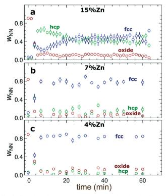
Fig. 6 Evolution of the relative concentrations of oxide, fcc-like and hcp-like phases, as obtained by the NN from operando Zn K-edge EXAFS data for bimetallic catalysts with a Zn loading of (a) 15%, (b) 7% and (c) 4% during CO<sub>2</sub>RR at a current density of -500 mA cm<sup>-2</sup>.
