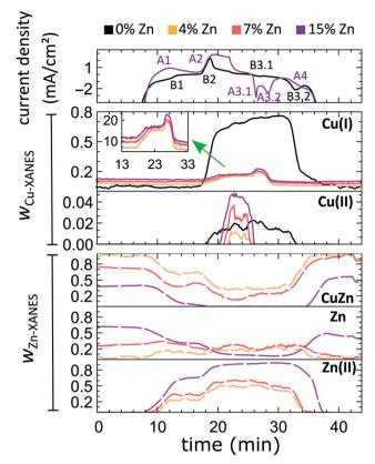
Fig. 8 Time-dependent changes in the current density during the CV scan, and the corresponding changes in the concentrations of Cu(ı), Cu(II), brass-like Zn and metallic Zn-like species with the current density plotted as obtained by the LCA of Cu K-edge and Zn K-edge XANES data.
