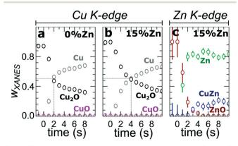
Fig. 4 Time-dependent changes in the weight of different Cu and Zn species, as derived from the LCA of XANES data collected during the  $\rm CO_2RR$  at -500 mA cm $^{-2}$  at (a and b) Cu K-edge and (c) Zn K-edge for the pure Cu<sub>2</sub>O NCs (a) and for the CuZn NCs (b) with a 15% Zn
