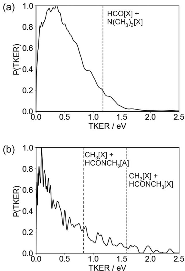
Fig. 7 Total kinetic energy release (TKER) distribution for the (a) N–CO and (b) N–CH<sub>3</sub> bond fission channels following 245 nm photolysis of DMF. The total available energies for the possible product channels are indicated by dashed vertical lines.
