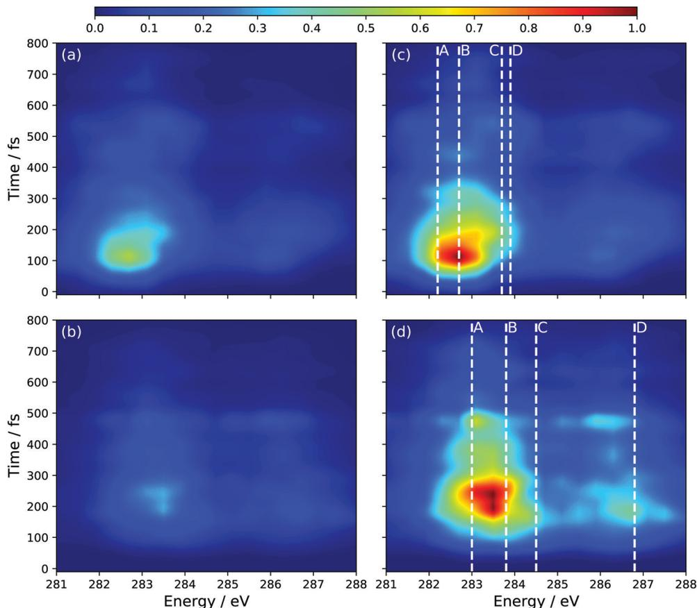
Fig. 7 Simulated  $S_1$  TRXAS at CVS-DFT/MRCI/aug-cc-pVDZ level of theory, decomposed into radicaloid (a) and polarized (b) contributions. (c) and (d) correspond to the intensity-renormalized plot of (a) and (b), respectively.
