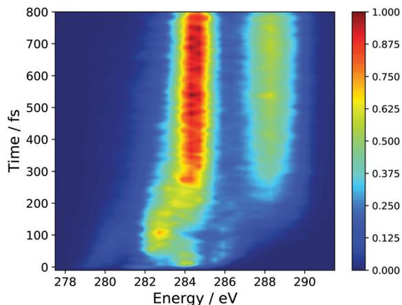
Fig. 5 Simulated TRXAS spectrum employing the results of AIMSD dynamics simulations and CVS-DFT/MRCI X-ray absorption cross-sections. An isotropic axis distribution was assumed.
