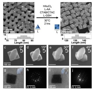
Fig. 2 SEM images of (a) tetrahedral Au seeds and (b) overgrowth product with histograms of nanocrystal edge lengths below. (c-f) SEM images of a single Au nanocrystal after overgrowth at tilts denoted in upper right. TEM images of overgrowth product along the (g) [100] and (i) [110] directions with representative tomographic reconstruction oriented to align with projection. Corresponding electron diffraction data in the (h) [100] and (j) [110] directions
