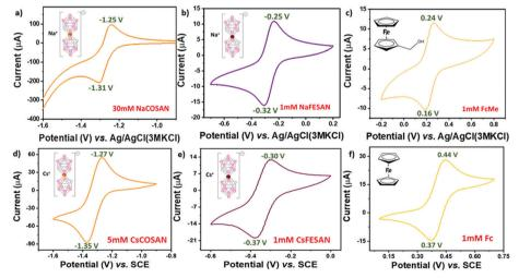
Fig. 2 Cyclic voltammograms for the reversible redox systems investigated with GC as the working electrode and Pt wire as the auxiliary electrode, measured at 100 mV s $^{-1}$ . (a) 30 mM Na[o-COSAN] in 0.3 M KNO<sub>3</sub>. (b) 1 mM Na[o-FESAN] in 0.3 M KNO<sub>3</sub>. (c) 1 mM FcMe in 0.3 M KNO<sub>3</sub>. (d) 5 mM Cs[o-COSAN] in 0.3 M TBAP/dry AcN. (e) 1 mM Cs[o-FESAN] in 0.3 M TBAP/dry AcN.
