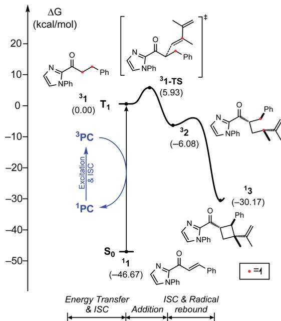
Fig. 9 Energy profile with triplet energy transfer mechanism.
