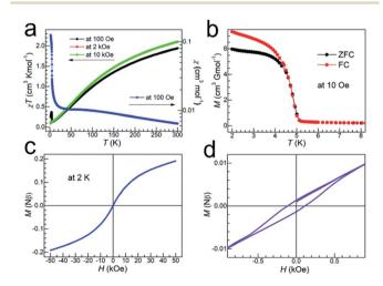
Fig. 3 Magnetic properties of TMCM–CrCl<sub>3</sub>. (a) Temperature dependence of the magnetic susceptibility ( $\chi T$ ). (b) Zero-field-cooling and field-cooling magnetization (M) under 10 Oe fields. (c) Field-dependent isothermal magnetization (M) at 2 K. (d) The zoomed views of magnetic hysteresis from (c).
