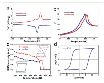
Fig. 2 Physical properties of TMCM–CrCl<sub>3</sub>. (a) DSC curves in heating and cooling runs. (b) The real part ( $\varepsilon$ ') of dielectric permittivity as a function of temperature. (c) Temperature-dependent SHG response in the heating and cooling runs. (d) P–E hysteresis loop measured along the polar axis of LTP at 373 K and 50 Hz.
