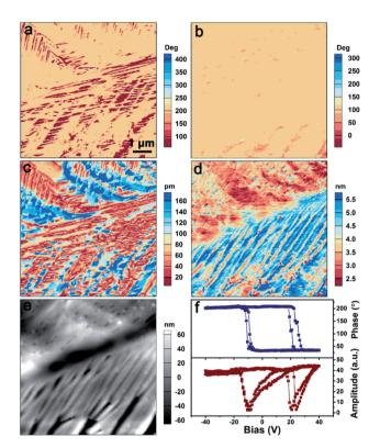
Fig. 4 Vertical PFM phase (a) and amplitude (c) images, lateral PFM phase (b) and amplitude (d) images, and topography (e) image of the thin film of TMCM–CrCl<sub>3</sub>. (f) Vertical PFM phase and amplitude signals *versus* the tip voltage for a selected point, displaying local piezoelectric hysteresis loops.
