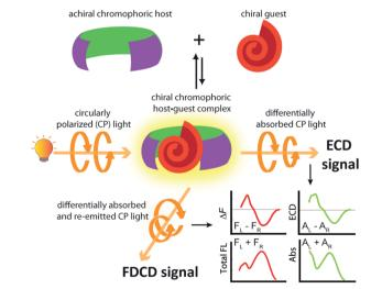
Fig. 1 Complexation of a chiral guest by an achiral chromophoric and emissive host can induce ECD and FDCD signal generation. The ECD signal measures the difference in absorption of left-handed and right-handed circularly polarized light by the chiral species whereas FDCD reports on the differential fluorescence intensity that results from excitation with left-handed and right-handed circularly polarized light.
