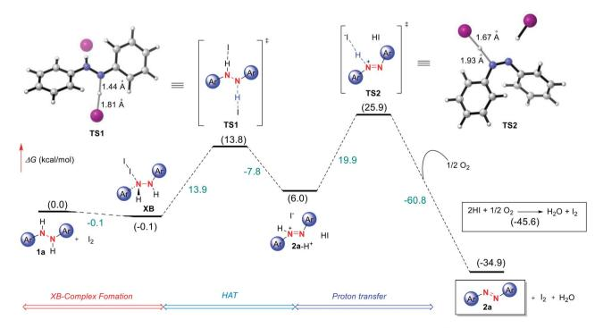
Fig. 3 Free energy profile for  $I_2$  catalyzed azo formation computed at the (IEFPCM<sub>DCM</sub>)UAPFD/def2-TZVP//UAPFD/DGDZVP level of theory. Free energies are given in kcal mol<sup>-1</sup>.
