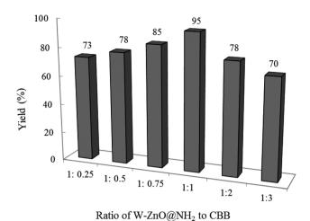
Fig. 11 Effect of  $W-ZnO@NH_2$ : CBB ratio on the efficacy of condensation reaction. Reaction condition is similar to that in the caption of Fig. 8. Reaction time was 2 h. 0.02 g of photocatalyst was used in all cases.
