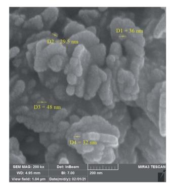
Fig. 19 FESEM images of the final reused photocatalyst.
