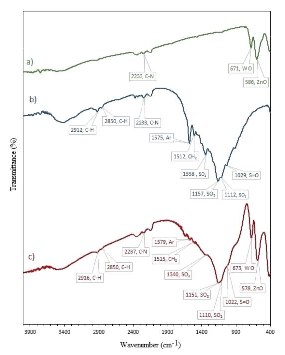
Fig. 1 FT-IR spectra of (a) W-ZnO@NH<sub>2</sub>, (b) CBB and (c) W-ZnO@NH<sub>2</sub>-CBB.
