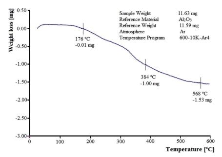
Fig. 4 TGA profile of W-ZnO@NH2-CBB nanocomposite.
