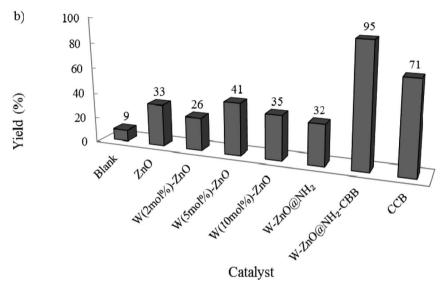
Fig. 8 Effect of different photocatalysts on the reaction progress. Benzyl alcohol and o-phenylenediamine selected as the starting materials and reactions were performed under an open atmosphere at room temperature in ethanol (10 mL) using an HP-Hg lamp for 2 h. 0.02 g of photocatalyst was used in all cases.
