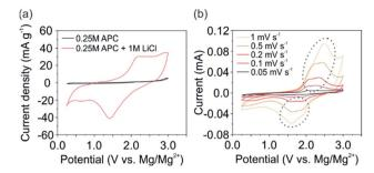
Fig. 2 Comparison of the electrochemical performance of 2<sup>nd</sup> CV cycles of a  $V_2O_5$  cathode at a scan rate of 0.1 mV s<sup>-1</sup> (a) using the APC and APC + LiCl electrolyte and (b) CV scans at different scan rates ranging from 0.5 to 1 mV s<sup>-1</sup>, using the APC + LiCl electrolyte.
