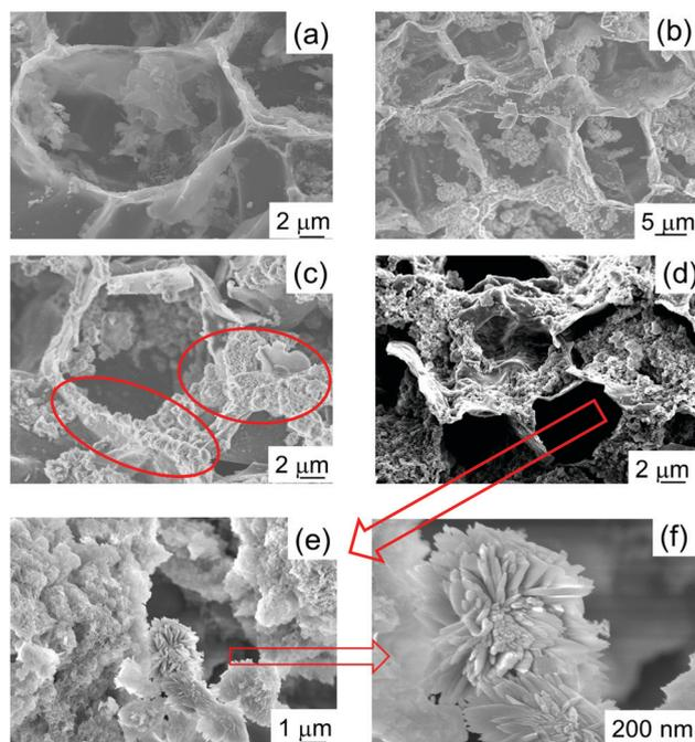
Fig. 2 SEM micrographs of HA samples prepared for different reaction times. (a) HA\_0:  $t = 0$  h; (b) HA\_4:  $t = 4$  h; (c) HA\_8:  $t = 8$  h; (d) HA\_16:  $t = 16$  h; (e and f) HA\_16 at higher magnification.
