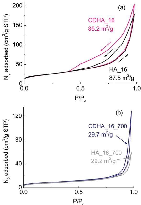
Fig. 5 BET adsorption and desorption isotherms for (a) HA<sub>16</sub> and CDHA<sub>16</sub>; (b) HA<sub>16\_700</sub> and CDHA<sub>16\_700</sub>. The numbers on the graphics indicate the values of the specific surface area of each sample.
