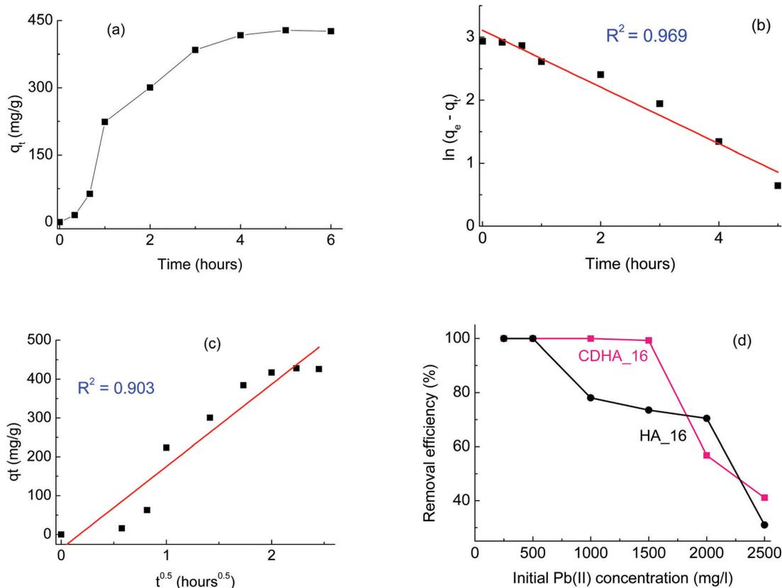
Fig. 6 (a) Kinetic study of Pb(II) adsorption by HA<sub>16</sub> with initial Pb(II) concentration of 2000 mg l<sup>-1</sup>; (b) and (c) fitting of the data with the Lagergren and Crank models, respectively; (d) removal efficiency for HA<sub>16</sub> and CDHA<sub>16</sub> with different initial Pb(II) concentrations.
