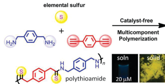
Fig. 7 Multicomponent polymerization for PTAM synthesis. The insets are the photographs of DMF solution and solids of PTAM taken under 365 nm UV light. Reprinted with permission from ref. 35. Copyright 2015, American Chemical Society.
