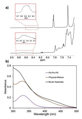
Fig. 4 (a) <sup>1</sup>H NMR spectroscopic overlay of (top) physical mixture of *co*-PIC and Pd-Pin-PS, and (bottom) assembled *co*-PIC-*brush*-Pd-Pin-PS after AgBF<sub>4</sub> addition. (b) UV-Vis traces of (purple) Pd-Pin-PS, (brown) physical mixture of *co*-PIC and Pd-Pin-PS, and (black) assembled *co*-PIC-*brush*-Pd-Pin-PS. (DCE, 25 °C).
