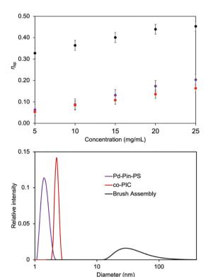
**Fig. 6** Characterizing the brush copolymer assembly by measuring (top) specific viscosity ( $\eta_{\rm sp}$ ) in CHCl<sub>3</sub> and (bottom) hydrodynamic radii ( $R_{\rm h}$ ) in DMSO; (red) **co-PIC**, (purple) **Pd-Pin-PS**, and (black) supramolecular brush assembly.
