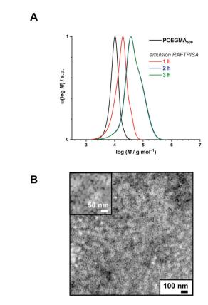
Fig. 2 (A) Size-exclusion chromatograms of polymers obtained by PBBMA emulsion RAFTPISA in water/ethanol 3:1 vol/vol at 70 °C with  $POEGMA_{500}$  at  $DP_{th}$  = 100, and 20 wt% solids content (entry 4 from Table S2†). (B) Transmission electron micrograph of nanoparticles obtained in the conditions mentioned above, after 2 h.
