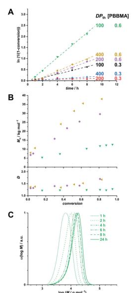
Fig. 1 RAFT solution polymerization of PBBMA in DMAc at 70 °C. (A) First-order kinetic plots for various [PBBMA] and DPth. Dashed lines correspond to linear fits. (B) Evolution of number-average molar mass (top) and dispersity (bottom) with PBBMA conversion for [PBBMA] = 0.6 M at various DPth. (C) Size-exclusion chromatograms of polymers obtained at different times for [PBBMA] = 0.6 M and  $DP_{th} = 100$ .
