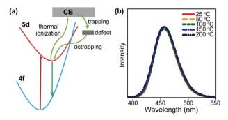
Fig. 8 (a) A simplified model for the zero-thermal-quenching due to structural defects. (b) Temperature-dependent emission spectra of  $Na_3Sc_2(PO_4)_3$ :Eu (divalent, 0.7%) phosphors under 370 nm excitation in the temperature range of 25–200 °C. Reproduced with permission from ref. 104. Copyright 2017, Nature Publishing Group.
