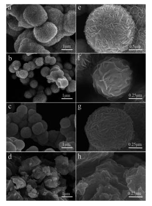
Fig. 2 (a and e) SEM images of  $220\text{-MoS}_2$ , (b and f) SEM images of  $200\text{-MoS}_2$ , (c and g) SEM images of  $180\text{-MoS}_2$ , (d and h) SEM images of  $160\text{-MoS}_2$ .
