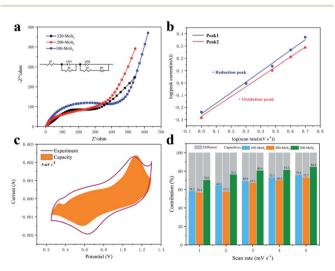
Fig. 7 (a) Electrochemical impedance spectroscopy of MoS<sub>2</sub> at different temperatures (inset is the equivalent circuit for fittings of the Nyquist plots of MoS<sub>2</sub>), (b) log(i) and log(v) curves of two peaks corresponding to the CV curves (200-MoS<sub>2</sub>), (c) capacitive contribution (orange) of 5 mV s<sup>-1</sup>, (d) capacitive and diffusion-controlled contribution ratios at multiple scan rates of MoS<sub>2</sub>
