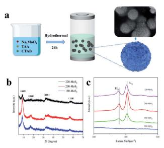
Fig. 1 (a) Schematic illustration of the preparation process of  $MoS_2$ , (b) XRD of  $MoS_2$  synthesized at different temperatures, (c) Raman spectra of  $MoS_2$  synthesized at different temperatures.
