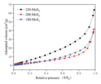
Fig. 3 Adsorption isotherms of MoS<sub>2</sub> at different temperatures.
