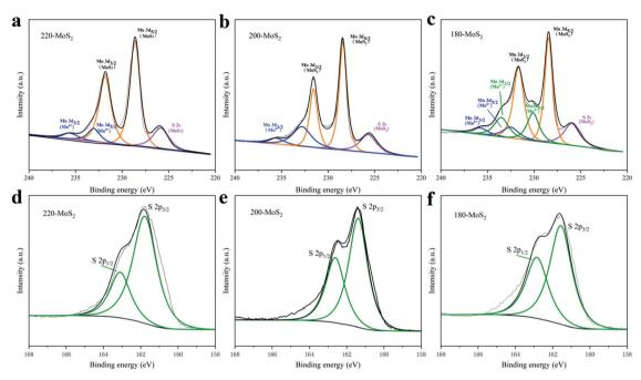
Fig. 5 (a–c) Mo 3d and (d–f) S 2s high-resolution XPS spectra of  $MoS_2$  prepared at different temperatures.
