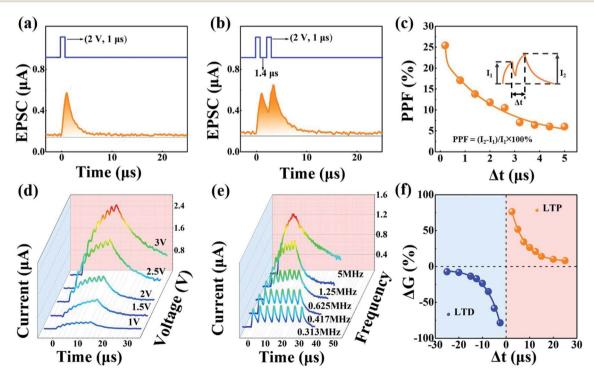
Fig. 5 Synaptic learning functions closely emulated in the Al/PVP–NCQD/ITO memristor. Short-term synaptic functions of (a) EPSC, (b) PPF, and (c) PPF versus the relative spike timing. A transition from STP to LTP appears through the (d) pulse amplitude and (e) pulse frequency. (f) Relative changes of the synaptic weight ( $\Delta G$ ) with spike timing ( $\Delta t$ ), showing the typical STDP function of the memristive synapses.
