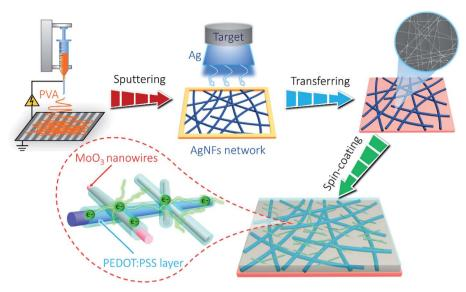
Scheme 1 The fabrication schematic of AMP film electrodes.
