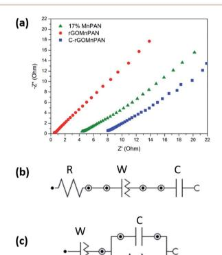
Fig. 7 (a) Nyquist plots of the 17% MnPAN, 1% rGOMnPAN and C-rGOMnPAN electrodes. (b) Equivalent circuit of the 17% MnPAN and C-rGOMnPAN electrodes. (c) Equivalent circuit of the 1% rGOMnPAN electrode.
