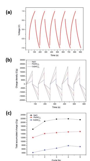
Fig. 8 (a) CCCD cycles in degassed 0.1 M KNO<sub>3</sub> using C-rGOMnPANdeposited graphene sheets as the working electrode, Ag/AgCl as the reference electrode and the Pt sheet as the counter electrode and (b) CDI performance using 100 ppm NaCl, 100 ppm Pb(NO<sub>3</sub>)<sub>2</sub> and 100 ppm Cd(NO<sub>3</sub>)<sub>2</sub> electrolytes; (c) salt removal capacity of the CrGOMnPAN electrode.
