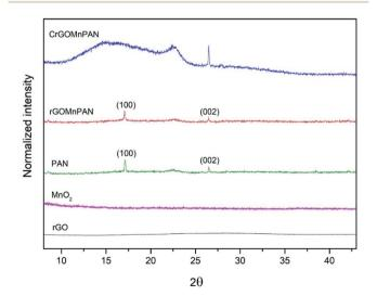
Fig. 2 X-ray diffraction patterns of rGO, the MnO<sub>2</sub> nanoparticles, PAN fibers, 1% rGOMnPAN fibers and C-rGOMnPAN fibers.
