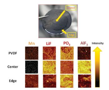
Fig. 4 Photograph of the negative electrode with 1 wt% polymer and TOF-SIMS images with and without 1 wt% polymer as a function of the analyze point position and the material detected.
