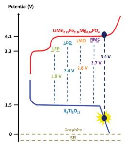
Scheme 1 Potential of the electrode materials used for constructing a full cell.
