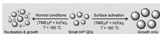
Fig. 11 (Fig. 1a in ref. 123). Two proposed reaction pathways for the growth of (InP) n quantum dots (QD) starting with the amine-based pre-synthesized seeds of InP QDs plus In(III) alkanoate, In(Fa) 3 (Fa = fatty acid carboxylate anion), and tris(trimethylsilyl)phosphine, (TMS) 3 P, in the absence (left) or presence (right) of the surface-activation reagent acetylacetone. Reproduced with permission from ref. 123. Copyright 2017 Springer.
