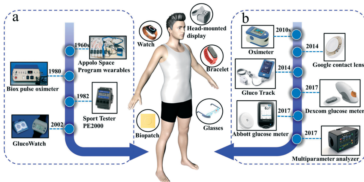
Fig. 1 The development of commercial translation for health monitoring wearable devices. (a) The past wearables for health monitoring. From the top: an initial prototype wearable equipment for astronauts in 1960s, an oximeter equipment worn on fingers in 1980, a watch-like wearable for heart rate monitoring in 1982, a wearable glucose meter based on iontophoresis in 2002. (b) The present advanced commercial wearable devices for patient-friendly diagnosis. From the top: a fingertip worn oximeter produced by Contec, Inc. (Hebei, China) in 2010s, Google contact lens for glucose biosensing and wirelessly transmitting signal in 2014, Gluco Track (Cnoga, Inc., Israel) as a finger clip for non-invasively monitoring glucose based on optical absorption and reflection in 2014, a G5 continuous monitoring wearable device (Dexcom, USA) for ISF glucose based on electrochemical platform in 2017, Abbott Freestyle Libre (Abbott, Inc.) for ISF glucose monitoring during 14 days by entrapping glucose oxidase on a soft conductive bio-needle in 2017, a fingertip analyzer produced by Cnoga, Inc. for multiplexed analysis based on optical absorption and reflection in 2017.
