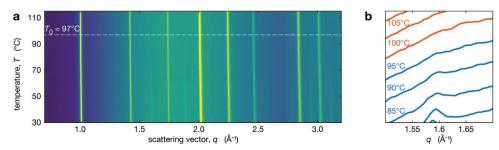
Fig. 2 (a) Temperature XRD map for  $Cs_{0.4}FA_{0.6}Pb(Br_{0.17}I_{0.83})_3$  with the extracted  $T_0$  (temperature where film is purely cubic) indicated by a dashed line. (b) Evolution of the integrated intensity of the t(210) superlattice peak. Temperature is increasing moving up in the vertical direction. The y-axis is linear and represents the intensity counts in arbitrary units.
